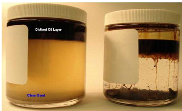
Figure 3 – Laboratory test comparison of modified enzyme treated (left) and non-treated (right) oil-water-sand mixtures.
